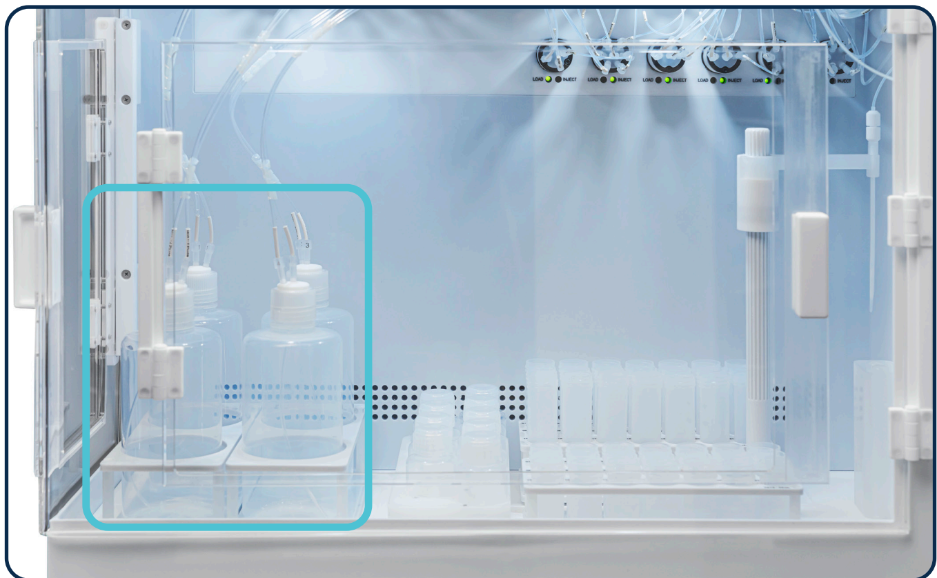
Layout of four 1 L enclosed bottle samples to the left of the autosampler.
